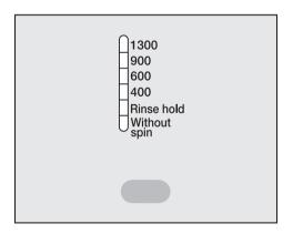
Press the "Spin" button repeatedly until the indicator light for the spin speed you want comes on. In some programmes the maximum spin speed is limited. The machine will not allow a higher spin speed to be selected.
